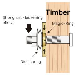
Magic-Ring tightens the bolt using the wedge principle
