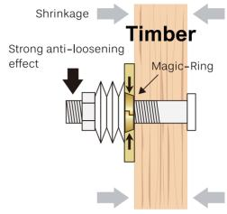
Even if the wood is thinned, the spring pushes in the Magic-ring and keeps the wedge effect and does not loosen
